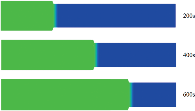
图 8 三个时刻(200s、400s、600s)的 PEGDA 凝胶溶胀变形图 Figure 8 Swelling and deformation diagram of PEGDA sample at 200s, 400s and 600s
